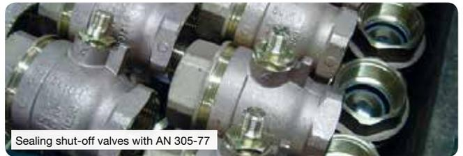
Sealing shut-off valves with AN 305-77
