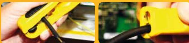
**Special tools for dismantling and stripping all common cables in the solar sector**
